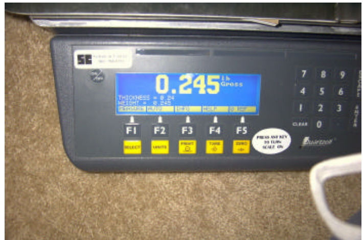
Close up view of scale display and keypad. Weight and volume capture is populated in to the DPS receiving screen fields speeding accurate data capture.
