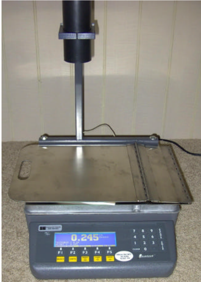
Full view Magazine "volume and weight" capture system. Magazines are placed inside the fold open metal sleeve. The overhead ultrasound device "bounces" signals off the top of the metal sleeve to capture magazine thickness.
